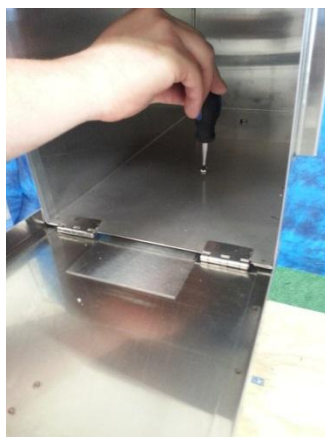
USE A SCREWDRIVER TO HOLD THE BOLTS IN PLACE
