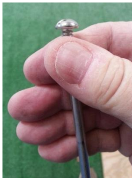
1/4" ROUND HEAD SS BOLT AT LEAST 3/4" LONGER THAN ARM THICKNESS
